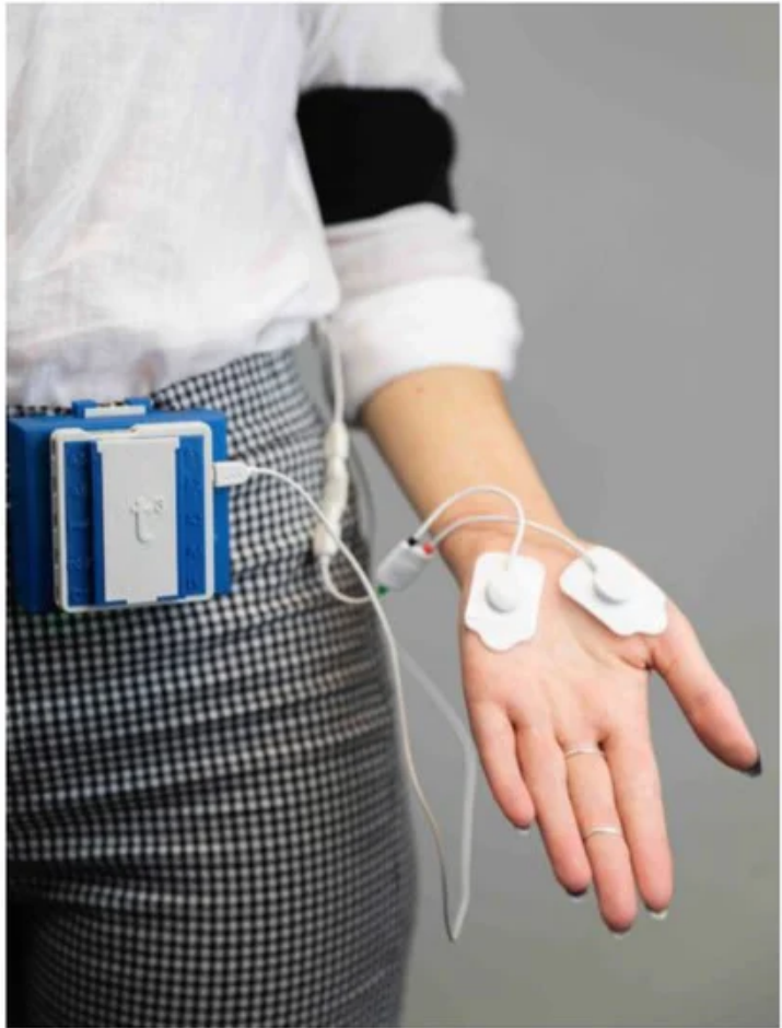
Fig. 3. The electrodes placed on the participant's non-dominant hand are connected to sensor cables wired to the COBALT Bluebox device.
