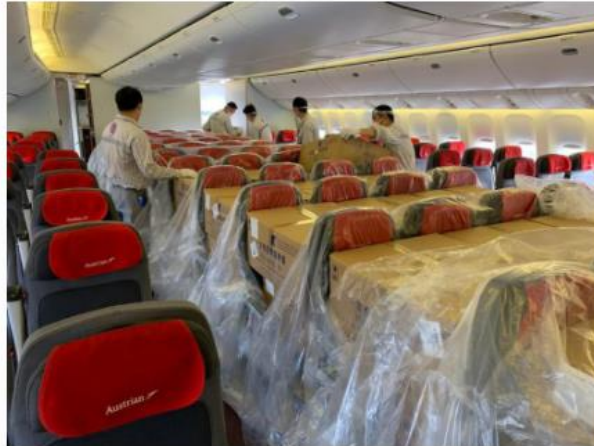
Austrian Airlines 777-200 being loaded with cargo in the passenger cabin. AUSTRIAN AIRLINES
