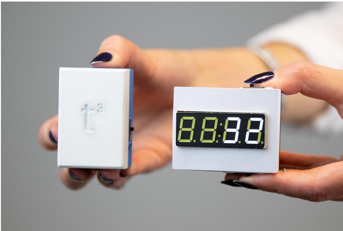
**Figure 2. Sync box (left) and light box (right) showing a number<sup>15</sup>**
