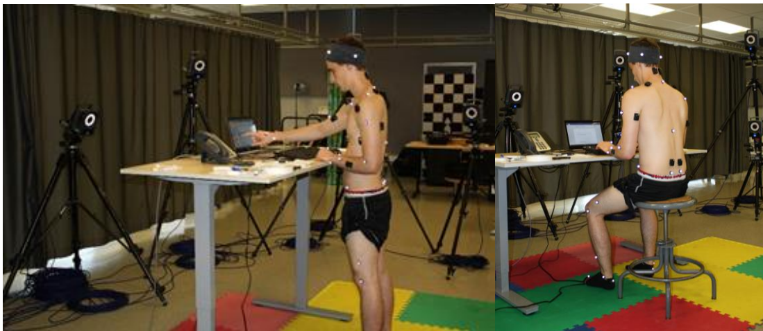
Figure 1: Experimental setup with reflective markers, EMG sensors applied on the skin of the participant in interaction with an active or seated desk
