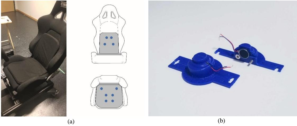
Figure 19. (a) A picture of the vibrotactile seat and a plan of the disposition of the mini vibrating motors on the seat cushion. (b) A picture of a closed shell with a mini vibrating motor inside (left) and the view inside the shell (right)
