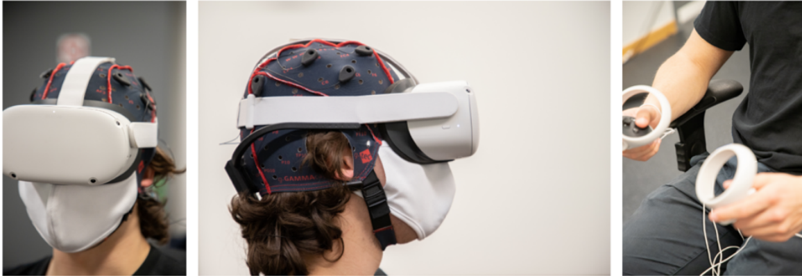
Figure 3. HMD combination of the EEG and VR headsets.
