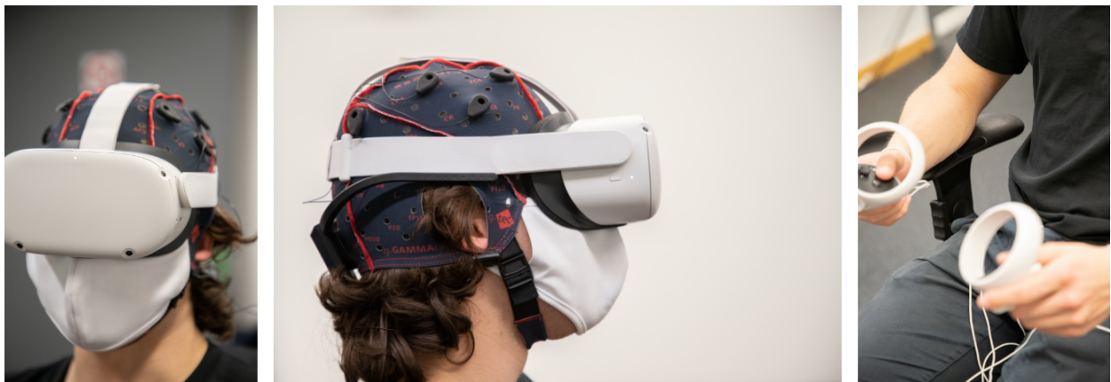
Figure 2.3 Combination of the EEG and VR HMD (left); VR controllers (right).
