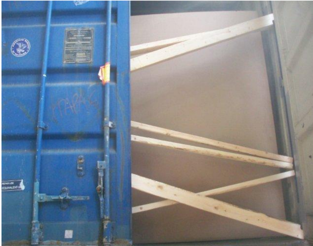
Figure 13 Loaded bulk container with retaining wall.
