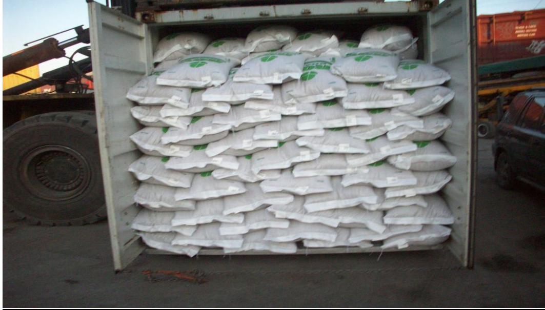
Figure 16 Container loaded over capacity with a plate
